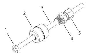
Figure 4: installation with screw-in unit
