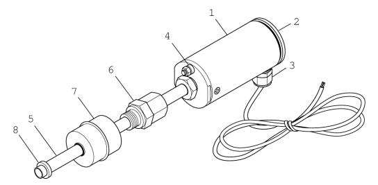
Figure 1: XT-1000 level sensor
