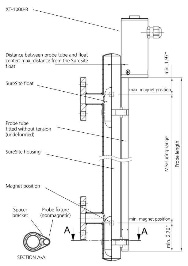
Figure 5: installation with SureSite
