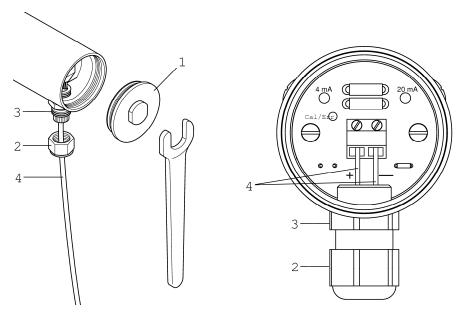
Figure 7: connecting the XT-1000 level sensor
