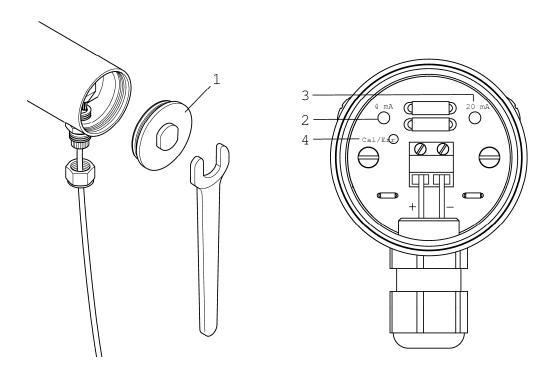
Figure 8: configuring the measuring span
