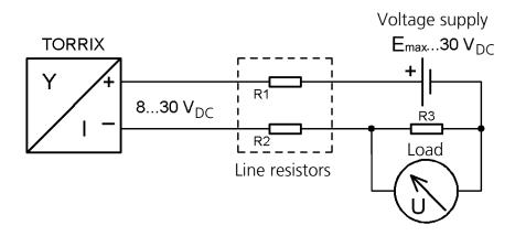
Figure 6: wiring diagram for XT-1000
