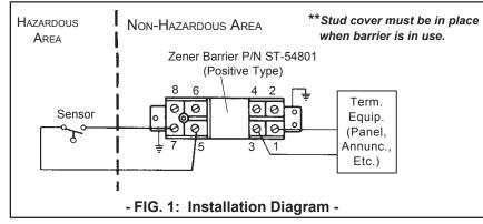
P/N 56750 Rev. P 5. Hazardous area field wiring will store energy due to distributed capacitance and inductance in proportion to its length. It is therefore recommended that the characteristics (available from the manufacturer) of the cable be known and judged against the length of run and atmosphere of exposure. The following chart is presented as a guideline in determining the limits of reactance for signal loops in the hazardous area wiring for this barrier.
