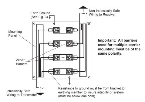
FIG. 2 Multiple Barrier Mounting
