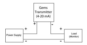
The 4-20mA current output circuit is designed to have current flow in one direction only **please observe polarity**. It is suggested that the cable shield be connected to the system loop circuit ground to improve electrical noise rejection.
