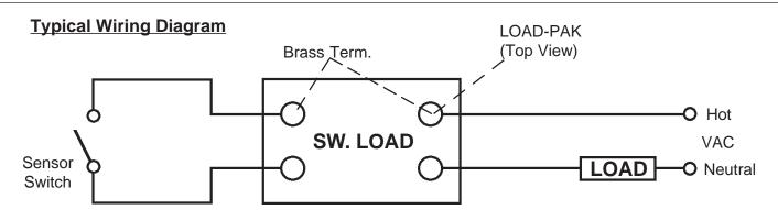
Wires connecting external sensor switches to LOAD-PAKS should not be placed in raceways or conduits containing high voltage lines. Voltages induced from these lines may trigger the low-power, solid-state triac; causing it to turn "on" momentarily.
