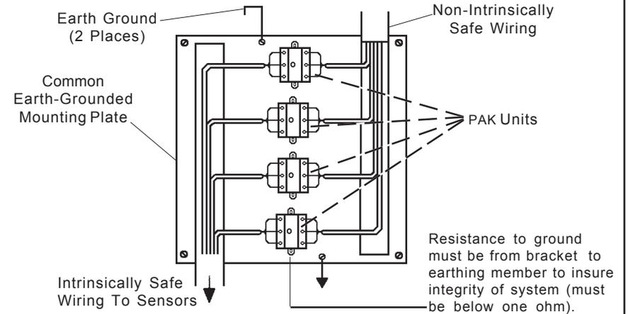
**Note:** All intrinsically safe wiring must be segregated from non-intrinsically safe wiring and shall have a minimum insulation thickness of .010".
